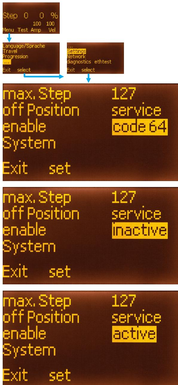
The connector for the high-resolution Gray code bit (see "Connecting") can alternatively be used to "enable" the code.
