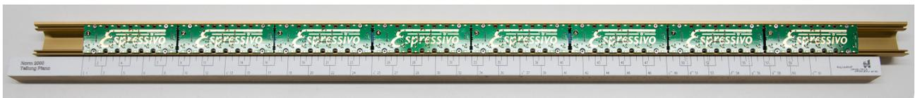
The sensor rail can now be tested: Connect the rail to the Master module (see below) and switch on the system. The LEDs of the modules (in the capital Espressivo E) flash for about one second after activation. If you approach a sensor position with a key magnet (ensure correct polarity) or a test pin (yellow tip), the LED of the respective sensor module lights up briefly.
