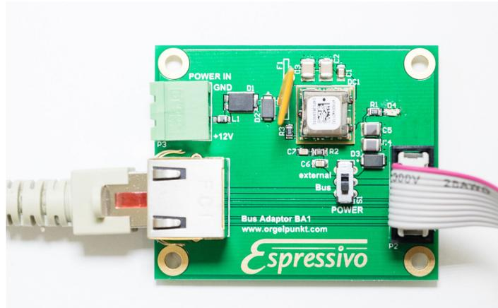
The earlier version of the bus adapter, BA-1, allowed for powering the pedal contact stock via the bus cable or external supply, alternatively. Always use the external power supply option. Tests have shown the power supply via bus cable to be unreliable depending on the cable brand. Make sure the “Power” switch is set to “external”. A red LED signals the presence of external power.
