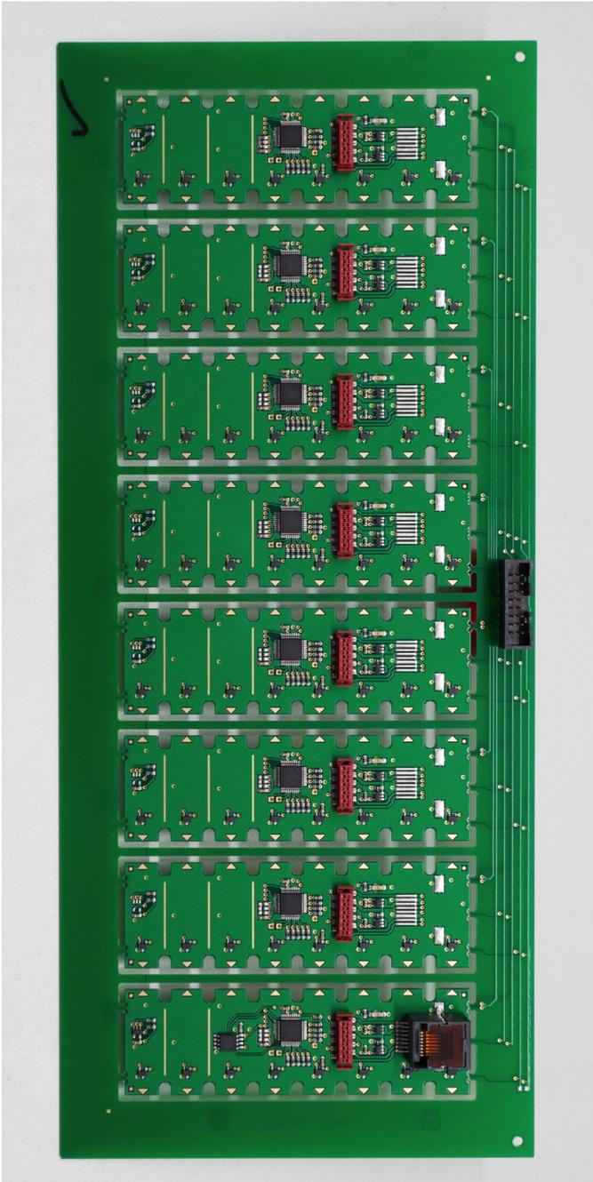
**The modules must not be connected to the Master module in their frame! The internal connections to the programming adapter on the frame cause short circuits in the voltage supply.**
