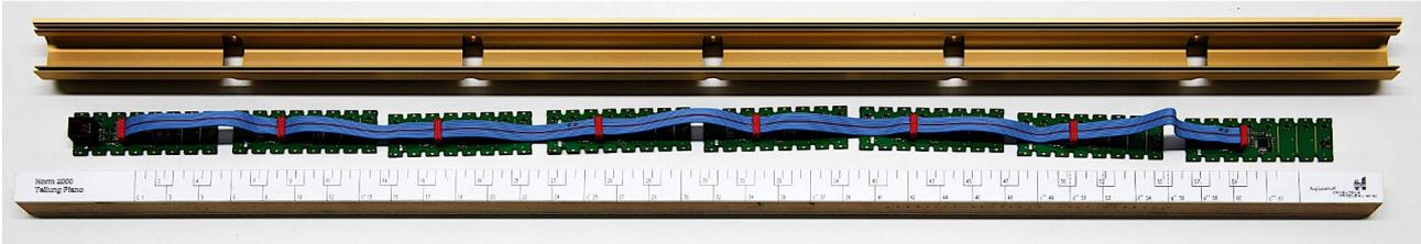
Align the gold triangle markers on the module edges to the manual scale and fasten each module to the profile with four screws. The modules should be flush with the rear profile edge.
