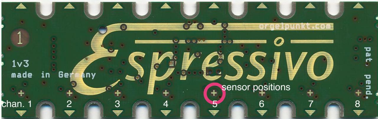
To fit different manual compasses, the sensor board(s) can be sawn off along the gold line ("cut here"). The cut lines should be as smooth as possible (file smooth) to prevent short circuits on the separated PCB tracks.
