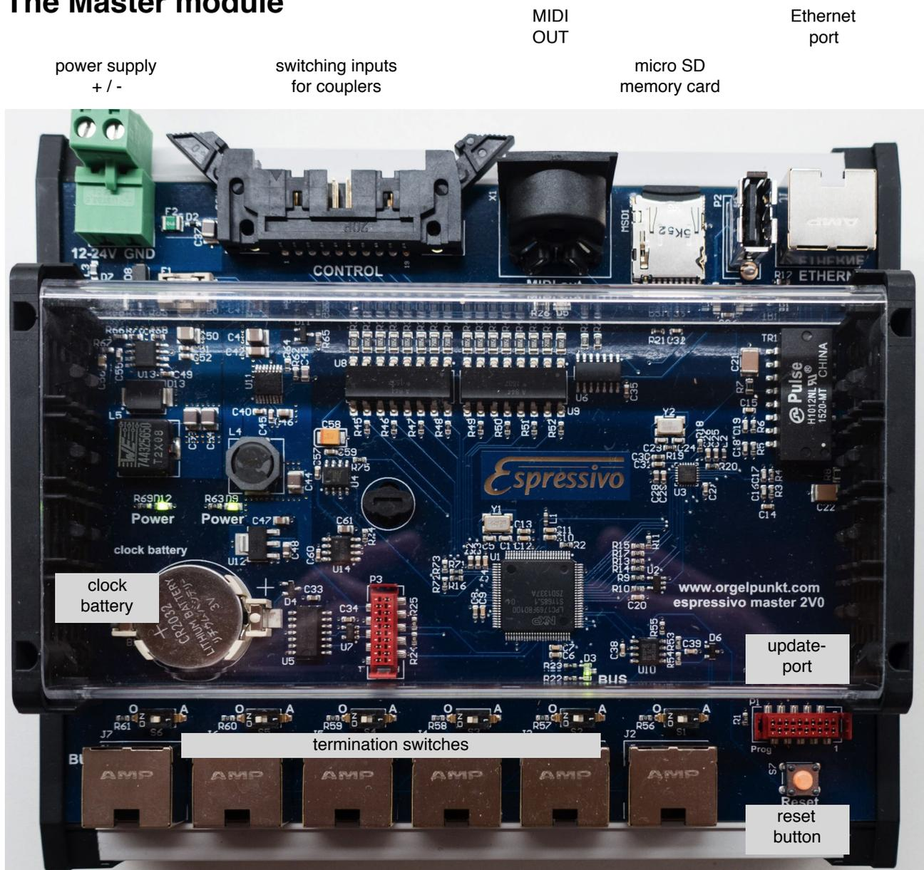
Up to six sensor rails or bus chains with individual sensors (up to two chains) can be connected to the Master module. The Master module powers the sensor modules, analyzes the data and generates the Midi signals that control the electric key action or other tone generators.
