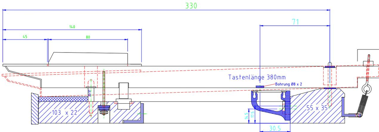
Always use the screws, washers and spring lock washers included in the packaging for fastening on the balance rail in order to guarantee permanent and stable connection between sensor strip and key frame. Unstable joints impair the switching precision when metal profile and wood move against each other.
