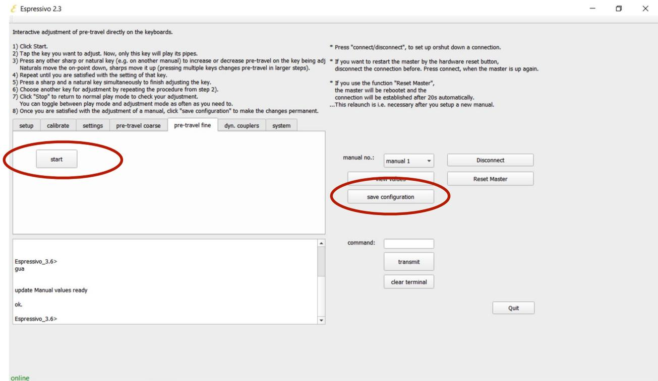
This function allows you to fine-tune and, at the same time, sound-check single keys on a fully assembled console. Mechanical and electrical action can thus be perfectly synchronized. This mode is recommended when individual settings need to be made by feel and ear, for example, to adapt the onset of the tone to the feel of a pressure point simulation.
