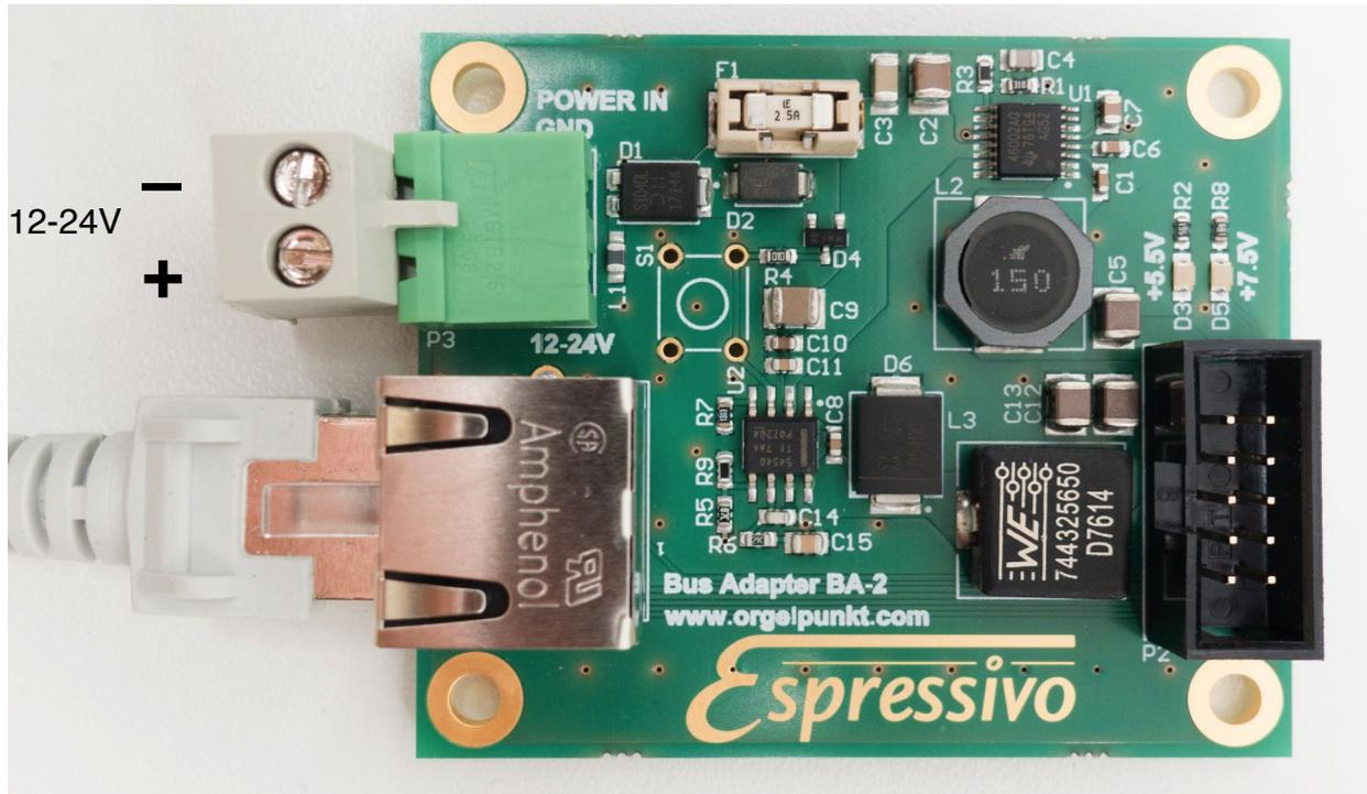
The pedal contact stock needs an additional power supply. Connect the bus adapter BA-2 to the same power supply (12 – 24V DC) used for the Master module (see p. 5). Two green LEDs signal the operation of the power supply circuitry of the BA-2.
