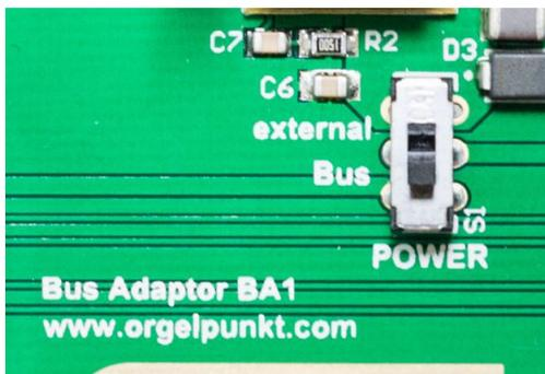
**The BA-1 adapter can only be used with 12V supply voltage, not 24V!**
