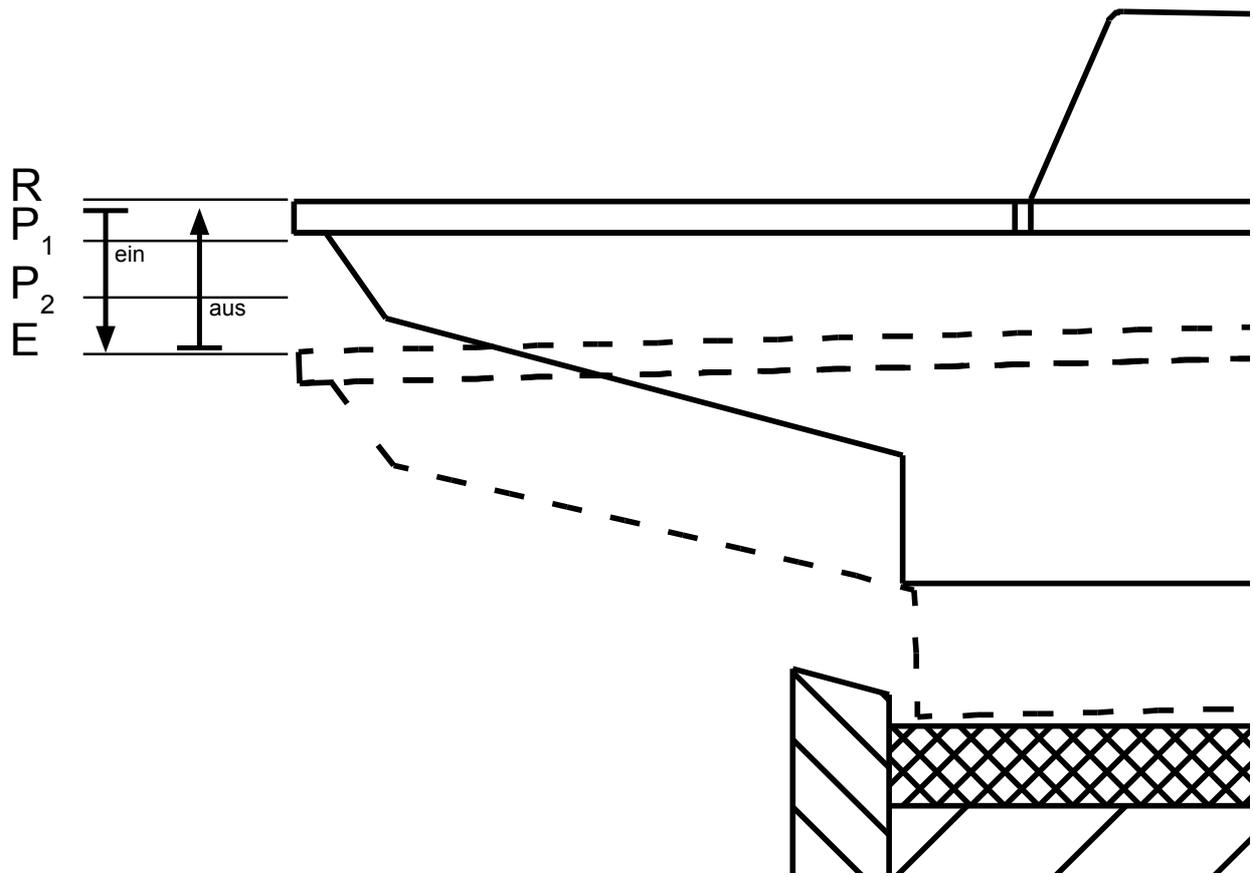
This positive hysteresis allows for a much better synchronization of mechanical and electrical action. In addition, any electrical action delays are compensated by premature switch-off.
