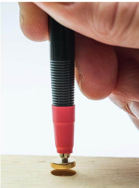
The correct magnet position can be easily checked with the positioning pin (red tip). The pin tip has a magnetic North Pole. As opposing poles attract one another, the key magnet attaches to the pin's South pole.
