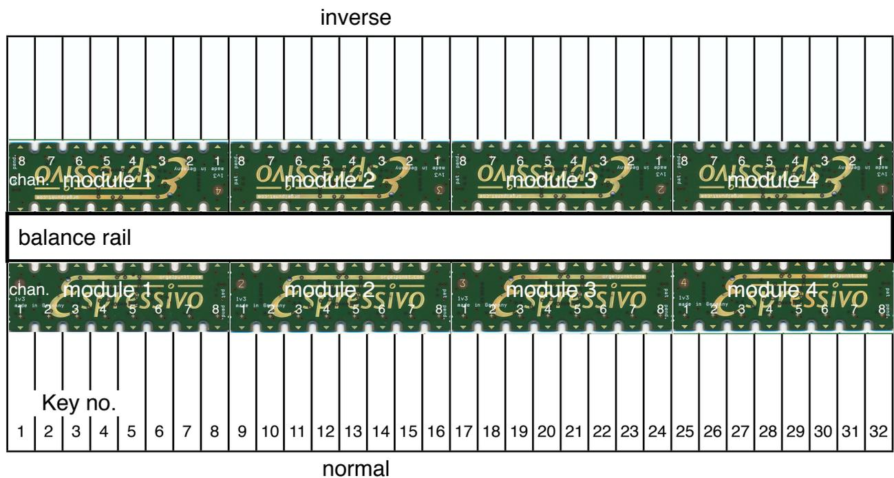
The system automatically identifies the type of assembly. The modules are always numbered consecutively from left to right. In case of inverse assemblies, however, the key sequence is opposite to the module numbers.
